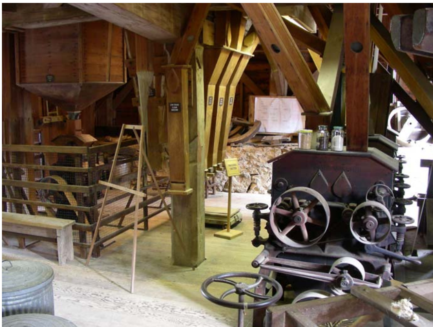
The three roller mills on the right made the bread flour from wheat. The miller bagged the flour at the chutes center.
