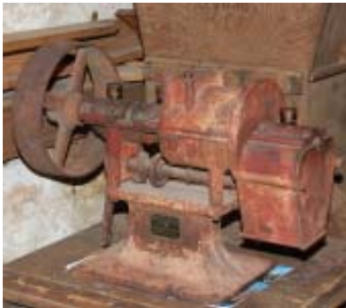
The buhr mill donated to us by Potter's Mill. When restored it could be used to grind meal at Pine Mills.
