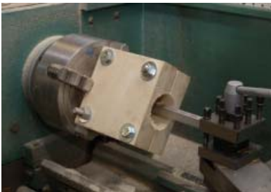
A very precise 2.700" hole that will accommodate the line shaft is being bored on David Metz's lathe in the hub block.
