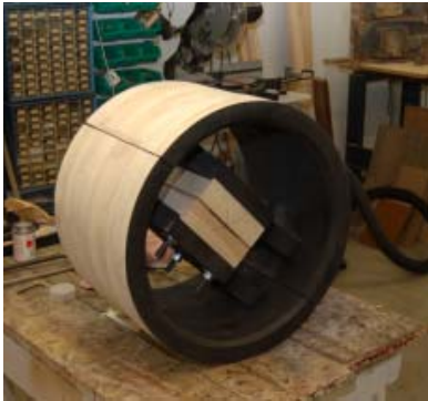
Our first wood flat belt pulley built by Scott Gibbs. 18" in diameter X 12" wide.
