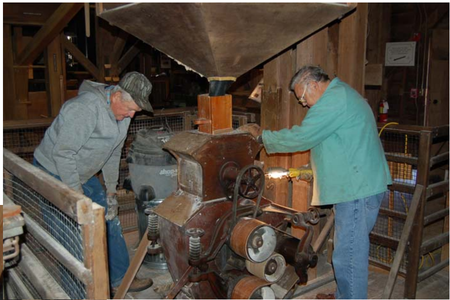
Joe Clark and Peter Allenger are unjamming our three roller corn mill. Once jammed it takes a careful cleaning to get it to run again.
