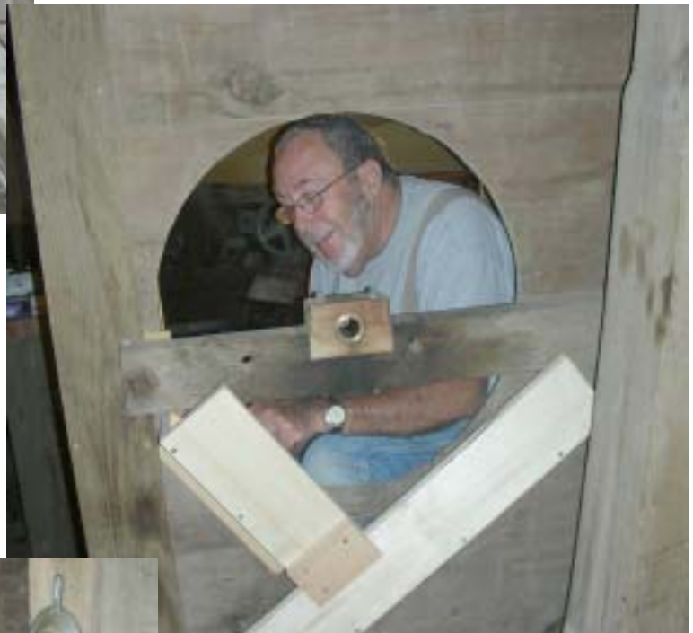
Yes, that's Bob Delong inside of the cottle collection bin! Bob had to climb inside (no easy task) to repair a rotted 2X4 brace. The cottle's rotating screen will take Bob's place after the machine's final assembly. The new boards in the "Y" shape collect any debris that tails-over the rotating screen.
