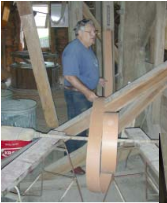
Yes, that's Bob Delong inside of the cottle collection bin! Bob had to climb inside (no easy task) to repair a rotted 2X4 brace. The cottle's rotating screen will take Bob's place after the machine's final assembly. The new boards in the "Y" shape collect any debris that tails-over the rotating screen.
